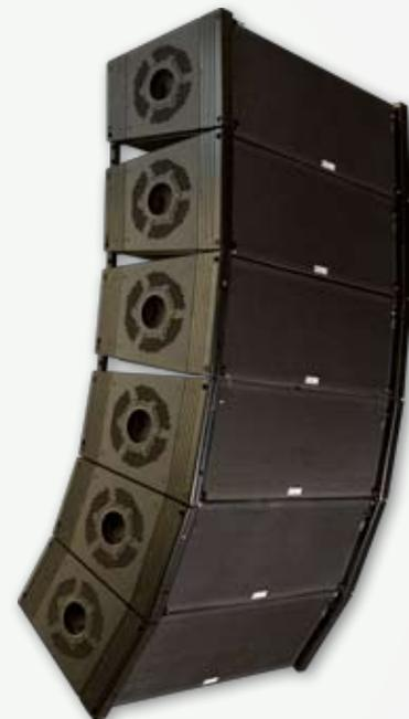
The lightweight extruded aluminum rigging of the KF740 allows for up to 16 enclosures at a 10:1 safety factor. EAW Resolution software defines the optimal array size and configuration based on venue dimensions.
