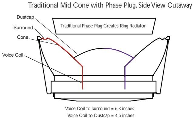
The distance from a cone driver's voice coil to its dustcap is shorter than the distance from the voice coil to either the cone or surround. Therefore, the energy radiating from the dustcap most often leads the energy from the rest of the system. Traditional phase plug designs have isolated this energy and routed it through a longer path than that which faces the energy from the cone or surround. In so doing, the phase plug attempts to equalize the arrival smear.
