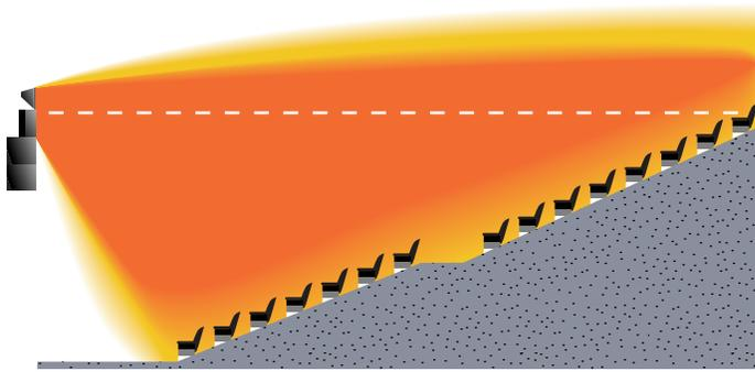
Since the vertical coverage pattern tilts downward, we recommend little or no downward horn aiming. Instead the system is aimed by elevation; the HF horn should be elevated to a height where it is directly in line with the last row of seats. This has been found to provide the best coverage front to back, and significantly simplifies setup and installation by removing the “guesswork” traditionally associated with horn-aiming behind the screen.
