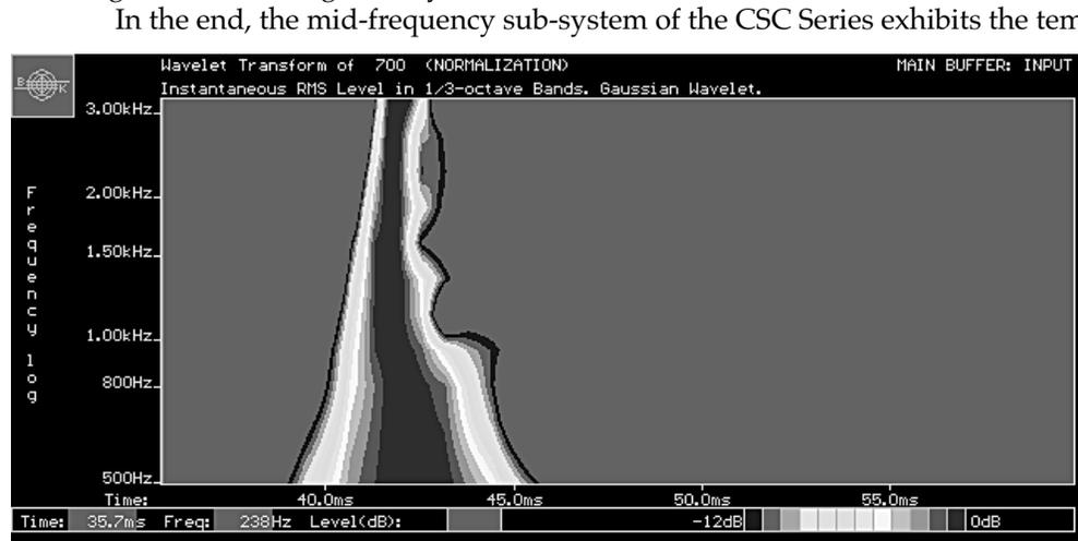
In the end, the mid-frequency sub-system of the CSC Series exhibits the temporal clarity of a compression driver alone (as in a two-way system) and the natural low distortion sonic reproduction of a cone transducer (as in an EAW three-way system) while removing crossover transitions from the vocal region and maintaining the spatial performance required for broad band constant directivity.
