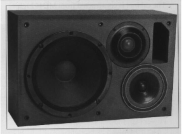
The low frequency section consists of an RCF L12/584 high efficiency driver mounted in a compact enclosure. The vent tuning is optimized for flat response and maximum output above 100 Hz. When used for all music reproduction applications, the DS123B is intended to work with a subwoofer system such as the EAW VB1 18 inch or VB215 dual 15 inch vented low frequency systems.
