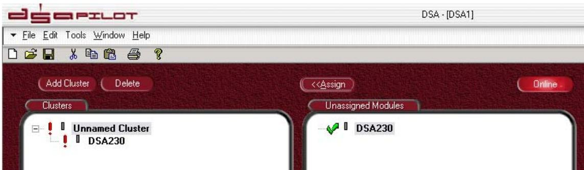
For example, if you were using a 1C cluster (single DSA230, LED at bottom), you would left click on the DSA230 in the 'Unassigned Module' window so it grays out, click on the 'ASSIGN' button, then left click on the DSA230 shown under the Unnamed Cluster, which is your 1C cluster.
