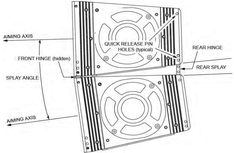
**NOTE:** Each SB730 Hinge Tube has only one hole for attaching the Hinge of another enclosure. As there is no choice of holes, it is neither labeled nor listed in the chart.
