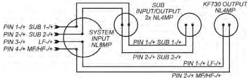
1. Connect the four different amplified signals needed to power a complete array of KF730s and SB730s to the SYSTEM INPUT.
