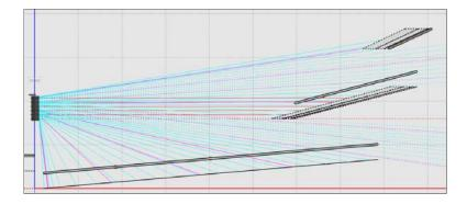
Whereas with a traditional mechanically-articulated line array, only a smaller number of cells (equal to the quantity of array modules) must be distributed across the entire seating cross-section. The array addressed by each cell, therefore, is very large:
