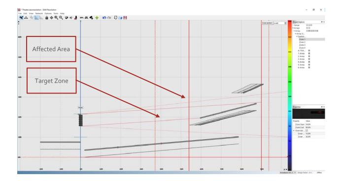
Once the user has selected their zone and entered the equalization parameters, the change will be live. If online with a system, the equalization will be applied to the output of the system. No parameter upload or additional calculations are necessary. Additionally, the effect of the Spatial EQ on the audience area SPL and frequency response will be recalculated and displayed.
