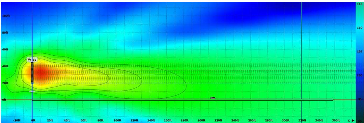
Below, a table relating array size, low-frequency pattern control and effective “throw” distance is provided as a rule-of-thumb guide. This assumes a flat audience surface and an array suspended at a typical trim height (i.e. approximately 10m/32 feet). More complex audience geometries will produce different results and should be studied in Resolution.
