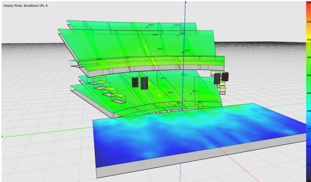
This example represents a typical 2,500-seat proscenium theater with a deep orchestra and under-balcony space, and a steep balcony reaching a height far above array trim. Two arrays of 6x Anna modules, and two arrays of 2x Otto can handle nearly any SPL application necessary for this venue. With an average of 105 dBA, the system is capable of reproducing high SPL program material to every seat in the house, without supplemental fills. This system also provides significant attenuation on-stage.
