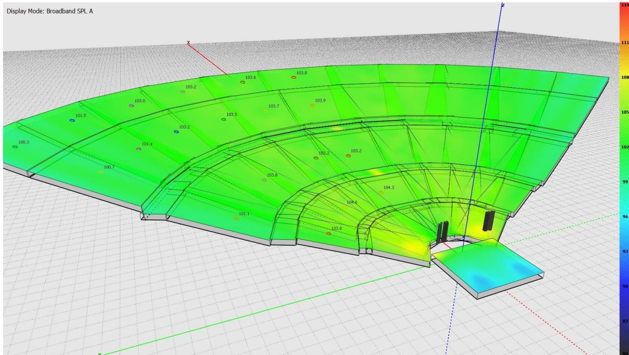
This example represents an outdoor “shed”-style venue, including a heavily-raked seating bowl and capacity of approximately 20,000 attendees. The system utilizes two arrays of 18x Anna modules each, and two arrays of 8x Otto modules each.
