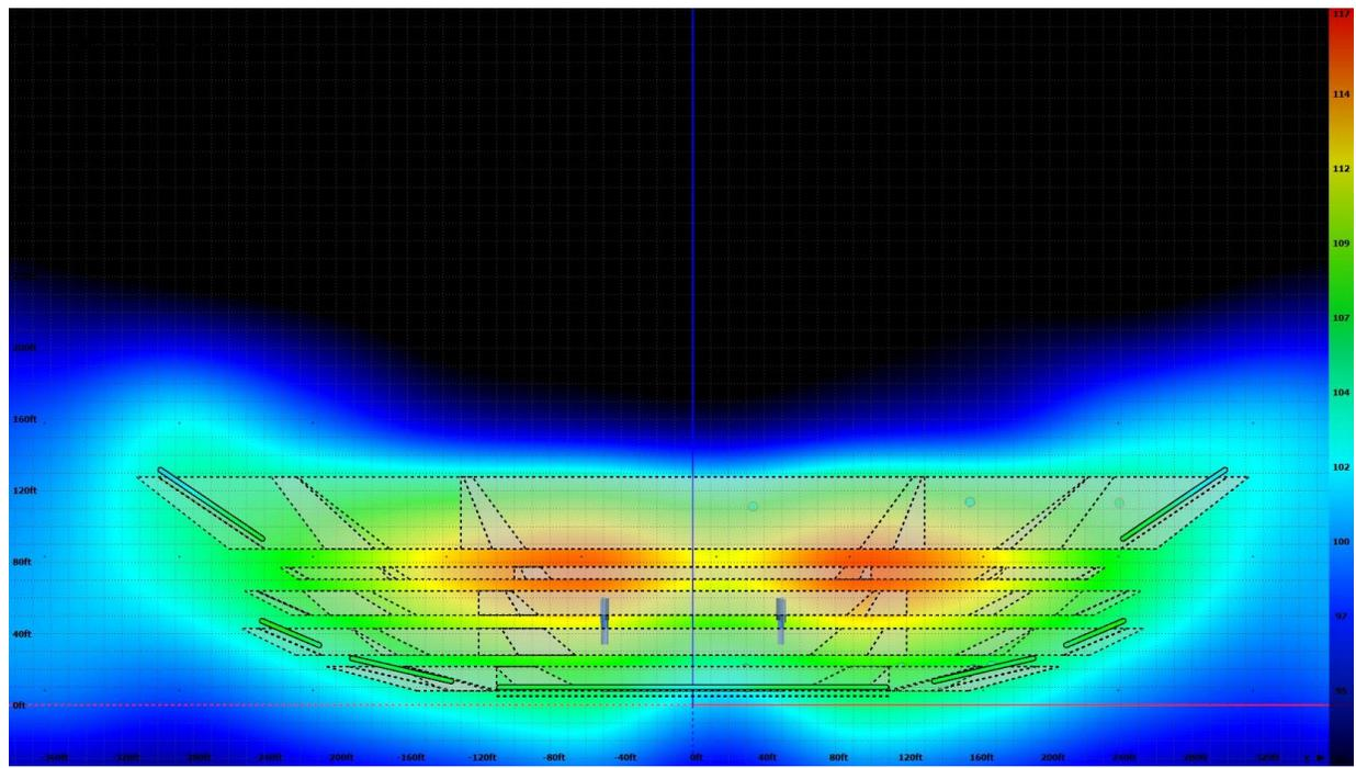
low frequencies. With Adaptive systems, the array's total output is available wherever coverage is defined. In the examples below, both 'full-coverage' and 'reduced-coverage' options are presented. In the 'reduced-coverage' scenario, SPL in the coverage zone is increased because the entire array is now being applied to a smaller area.
