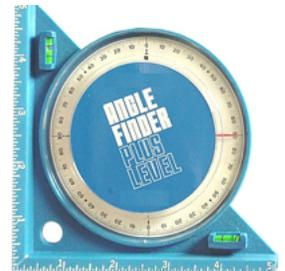
Place the angle finder against one of the rigging tubes on the face of the uppermost enclosure in the array that can be physically reached. Adjust the angle of the entire array so that the face of this enclosure is set at its prescribed aiming angle listed in Resolution.
