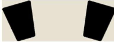
The optimum spacing in most applications when using two MicroWedges. The wider spacing (approximately two MicroWedges) greatly increases the side-to-side width of the “sweet spot” while maintaining the increased volume realized with two wedges. Additionally the “stereo sounding” effect of having two sources will be more apparent as the distance between the MicroWedges is increased.
