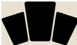
This configuration is extremely effective in producing substantial low-frequency energy while maintaining a very high level of vocal clarity and volume. Like the triple MicroWedge setup above, instruments are usually sent to the center wedge mix and vocals to the outside monitors.
