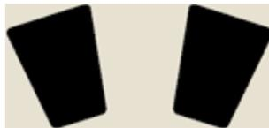
In applications where more volume (than provided by a single wedge) is required, and where keeping the coverage of the mix localized is preferred. The “sweet spot” will be fairly narrow from side to side, and applies mainly to covering a stationary performer. The distance between the wedges is equal to one MicroWedge.
