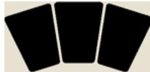
This is an exceptionally effective setup that maximizes the advantages of the trapezoidal angle design of MicroWedge Series cabinets. Vocals are usually run to the outside monitors, and the instruments to the center wedge. There are several advantages achieved by separating the instruments from the vocals, including improved coverage and clarity.
