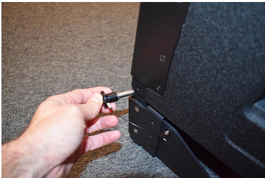
Figure 54 – Pinning RSX212L to frame in a ground-stack array
