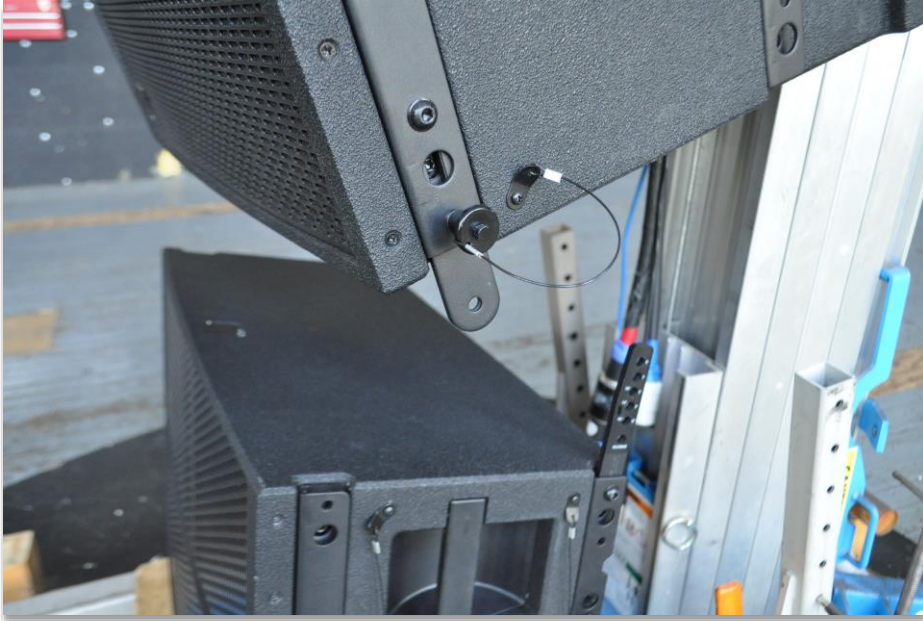
Figure 30 - Rigging tabs pinned into place to allow for insertion into the front rigging tube of the lower loudspeaker
