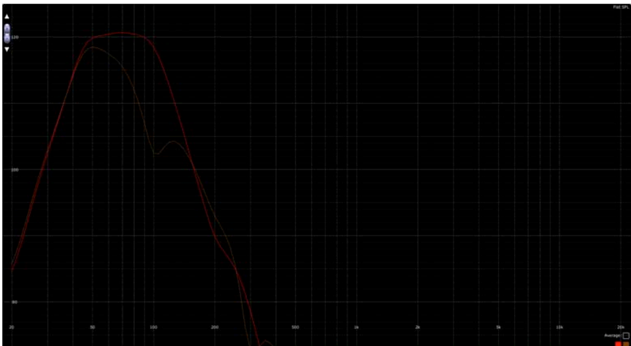
Figure 13: Frequency response at equal distances in and front (red) and behind (brown) 'quasi-end-fire' array.
