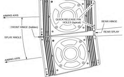
**NOTE:** Each SB730 Hinge Tube has only one hole for attaching the Hinge of another enclosure. As
