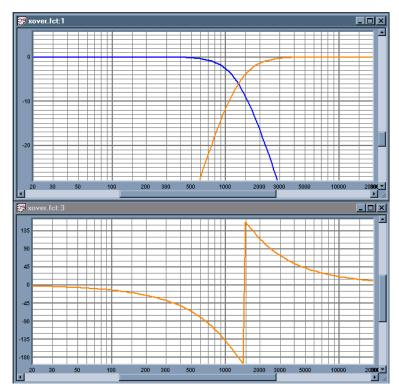
Figure 8: 24dB L.R. HPF and LPF, both at 1.3kHz. Note that the phase responses overlap, so the blue phase plot is not visible.
