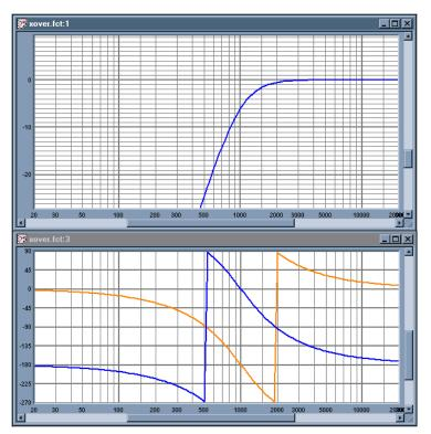
Figure 2: Two identical filters. Orange - normal, Blue - inverted polarity.
