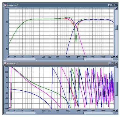
Figure 11: System shown in Figure 10 with crossover point set to 1.8kHz. Red – with 0.5ms delay, Green – without delay.
