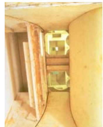
EAW's proprietary construction techniques combine high density polyurethane foam and thin, flexible sheets of laminated birch to produce large complex horn flares that are acoustically rigid.
