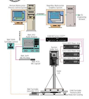
every system (72 points for each horizontal polar [0° to 355°] x 37 vertical polar angles [0° to 180°] x 29 third-octave centers).
