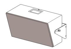
**WARNING:** Installation should only be done by an experienced technician. Improper installation may cause serious injury. The surface where the bracket/cabinet is to be fastened must have enough structural integrity to support 250 pounds.
