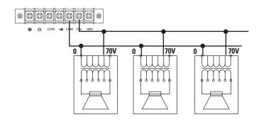
COM and 100V are used to connect 100V speakers Use Class I wiring:
