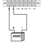
The unit can be powered using a 24 VDC power supply (if the rear panel DC POWER SWITCH is pressed in). This serves as a backup supply in case of an AC power failure. The unit seamlessly switches to the backup supply if there's a power loss, allowing safety instructions and emergency communications to continue. When both AC power and 24 VDC power are connected, the AC power is used and no current is drawn from the DC supply.
