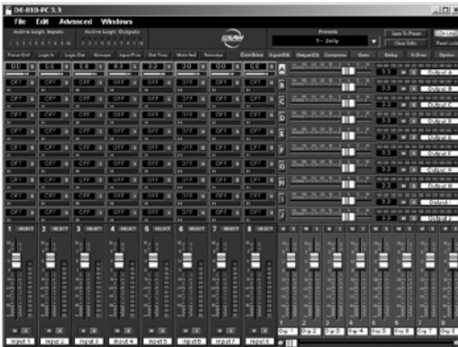
The main interface screen offers 8 input faders, 10 output faders, 80 crosspoint faders, and 32 group faders
