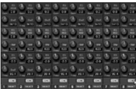
The input EQ view offers three filters for each input, with rotary gain and frequency controls for the High and Low Shelving filters, and gain, frequency, and bandwidth controls for the Bandpass filter
