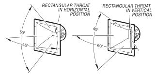
b. Reattach the horn assembly with the eight (8) flat washers, lock washers and screws removed in Step 2.
