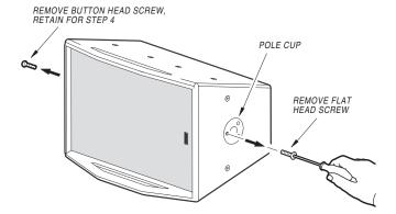
Remove the U-Bracket mounting hardware from opposing sides of the enclosure. Retain button head screw.
