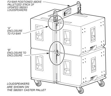
Rigging tubes, hinges, and their tethered quick disconnect pins are attached to both sides of the updated SB2001 Loudspeaker. These instructions apply to both the right and left sides of the Fly-Bar & Loudspeakers. To disassemble the array reverse the sequence of the operations defined in these instructions.
