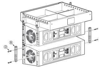
Attach the rear splay bracket through the hole combinations specified in Table 1 using two (2) 2-1/2 long screws (item D) per side. Before installing add a drop of Loctite 242 to the screw's threads. Hand tighten screws.
