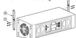
b. Loosely attach each Rear Splay Bracket (Item A) to the top, rear holes of the loudspeaker per Table 1 below, using one (1) 2-1/2" long screw (Item D) per side. Before installing apply a drop of Loctite. Do not tighten screws.
