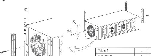
This table lists the desired splay angle, and the corresponding top and bottom loud-speaker rear attachment points. Angular settings not available are marked N/A.
