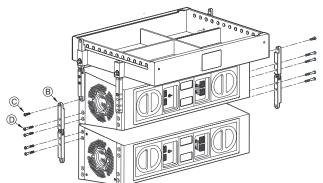
suspended loudspeaker using the two (2) 2-1/2 long screws (item D) and one (1) short screw (item C) per side as shown in the illustration. Before installing apply a drop of the user supplied Loctite 242 to the screw threads. Hand tighten screws.
