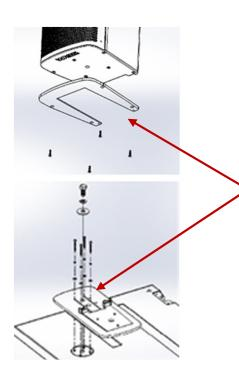
This kit includes everything needed to lock 1 AC6 onto a sub with a 20mm bolt in the pole cup.
