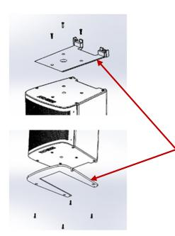
This kit is a top and bottom plate and allows 1 AC6 to be locked to another AC6. Note to "fly" you also need the stinger and mohawk
